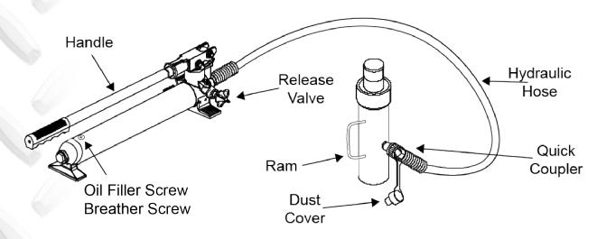
NOTE: When using this Porta Power Equipment always open the oil filler screw/breather screw
