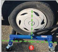
Tyre width, Diameter and Vehicle Gross weight are important factors to consider when using your TradeQuip Vehicle Positioning Jacks. For your safety you should not exceed the 680Kg Load Rating, 280mm Maximum tyre width and 750mm Maximum Tyre Outside Diameter.
