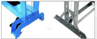
Once the press is positioned, we recommend using suitable fasteners to attach the press feet to your flat floor to prevent movement of the press during all operational procedures.
