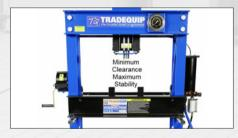
Always ensure that all compatible pushing adaptors supplied for the press ram have been correctly attached to the ram output shaft to provide lateral stability and prevent damage to the ram.
